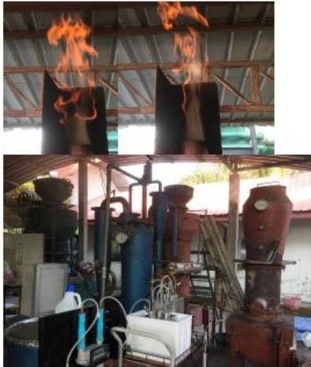
Flammability of producer gas
