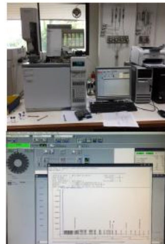
identification tar compound by GC-FID
